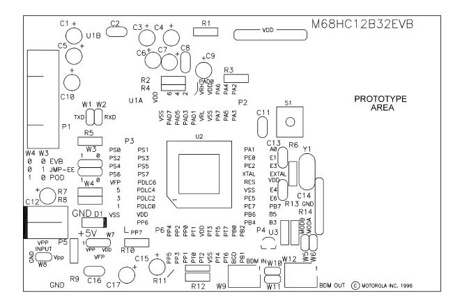
Figure 1-1. EVB Layout and Component Placement
